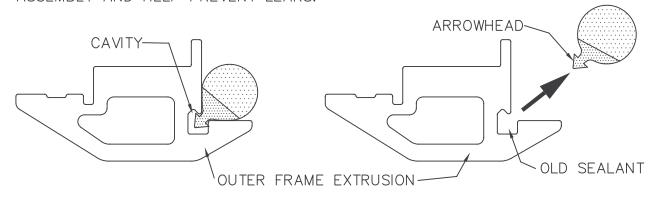
WHEN REFITTING THE SEAL IT IS IMPORTANT TO NOTE THAT THE SEAL IS NOT THE SAME ON BOTH SIDES, THERE IS A SLIGHT STEP WHICH APPEARS AS A LINE ALONG THE SEAL. ON ONE SIDE OF THE SEAL THE STEP IS FURTHER AWAY FROM ONE SIDE THAN THE OTHER. FIT THE SEAL WITH THE STEP FURTHEST FROM THE ARROWHEAD CLOSEST TO THE CENTRE OF THE PORTLIGHT.
